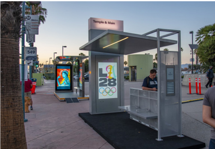
Digital signage with real-time arrival information and lighting
